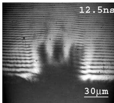
Fig.1 Shadowgraph of the plasma plume after the action of laser pulse with energy of 200uJ.
