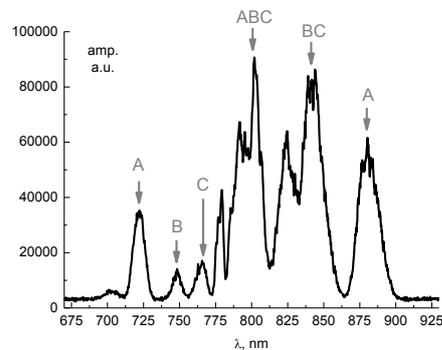
Fig.2. Example of the pulse spectrum inside the filament (molecular nitrogen at 0.96 atm, aperture size – 500  $\mu\text{m}$ , propagation length – 235 cm).
