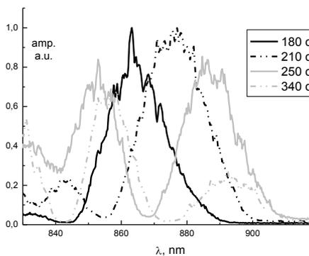
Fig.1. Transformation of the spectral intensity distribution with propagation distance (molecular nitrogen at 0.96 atm, aperture size – 500  $\mu\text{m}$ ).
